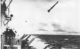
Rocket-boosted weapon is launched from destroyer after attaching to control system for ejection data from ship's own guns.
